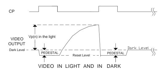
Figure 3. Definition of the Video Pixel in the Light and in the Dark
