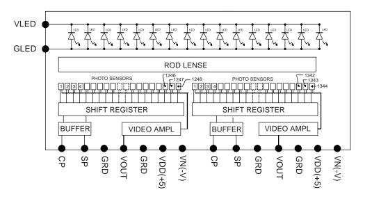
Figure 1. PI324MC-A4 module block diagram. (See Table 1 for pin-out designation)
